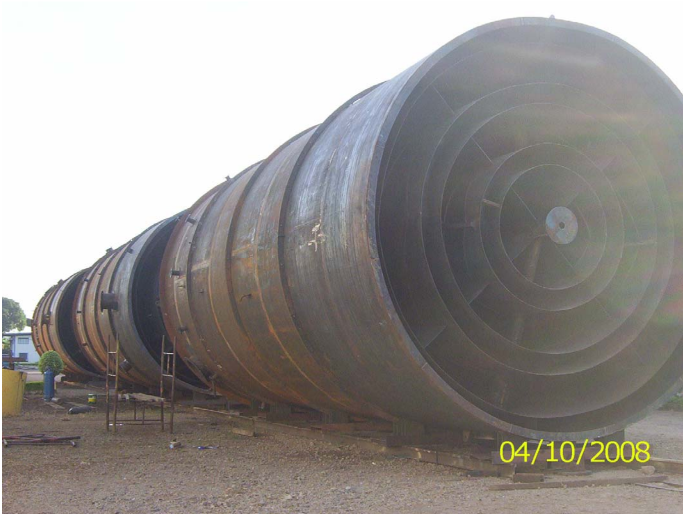
CPT Inc. six (6) meter diameter and fourteen (14) meter high column in sections
