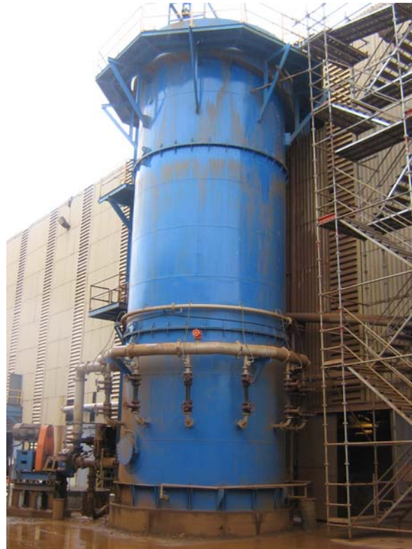
Figure 2 CPT Flotation Column fitted with Cavitation tube sparging system
