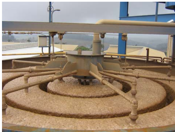
Figure 3 CavTube generated froth
