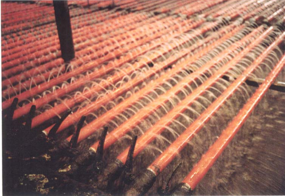
Figure 2: The use of wash water improves concentrate quality
